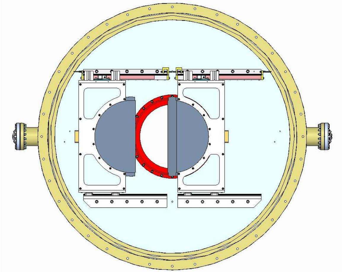
Figure 1: Drawing showing the shield assembly.
