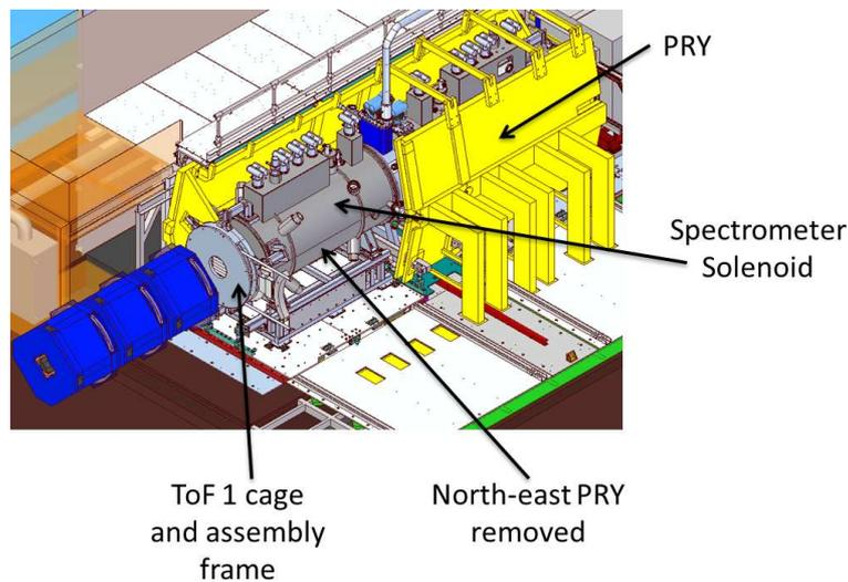
Figure 7: PRY around TOF1 and spectrometer solenoid. [6]
