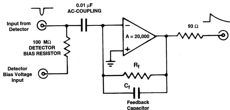
Figure 4: Simplified Schematic of the ORTEC AC-Coupled Charge-Sensitive pre-amplifier. (For a dc-coupled pre-amplifier, the detector bias resistor is removed, and the 0.01 μF capacitor is replaced by a wire. [4])
