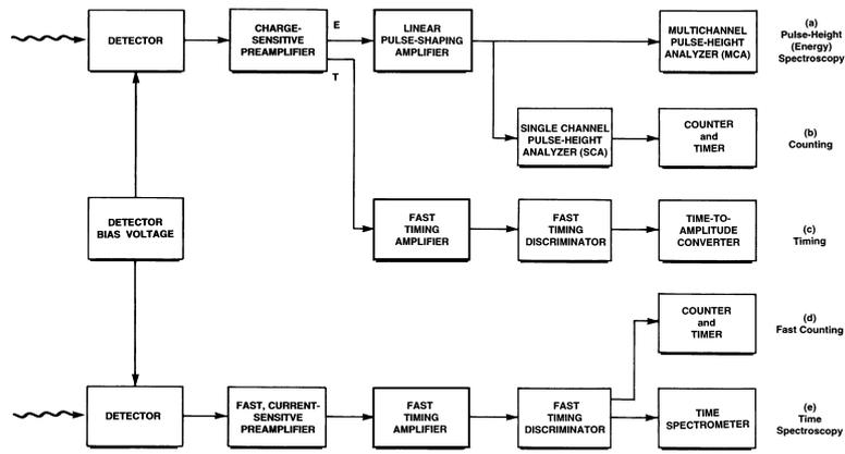
Figure 5: Typical Amplifier Applications in Pulse Processing. [5]
