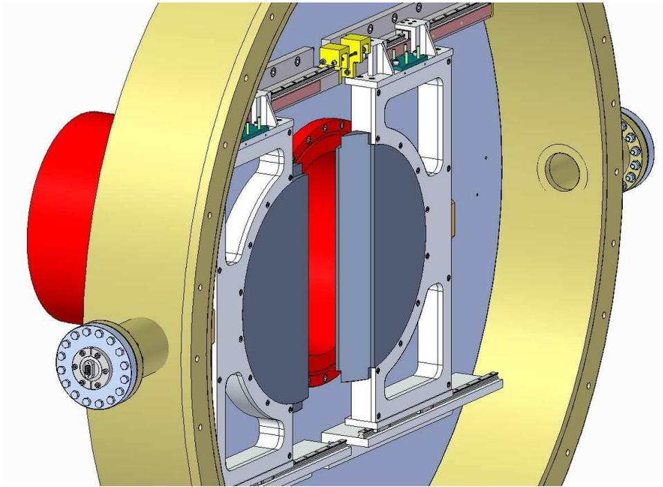
Figure 3: Drawing showing the sheild in close up.
