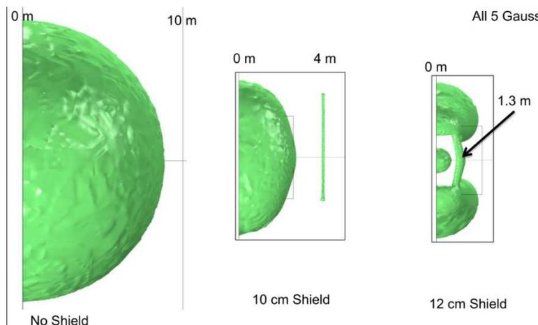
Figure 6: 5 G iso-surface plot of MICE for the 200 MeV flip mode, shielded and unshielded, in frontal view. [6]
