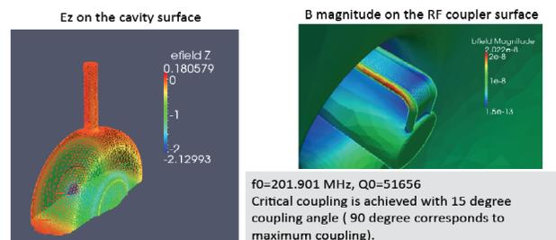
Figure 2: Omega3P simulation results: the left figure shows the  $E_z$  field on the cavity surface, and the right figure shows the B field in the coupler region, where the peak B field is located.
