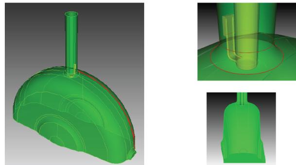
Figure 1: The RF model of MICE 201 MHz cavity, built from the CAD drawing. The left figure shows the half cavity geometry that we simulate, the upper right shows the RF coupler region and lower right features the curved Be windows on both sides.
