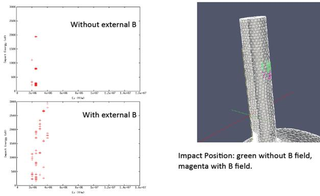
Figure 6: The MP in the coaxial waveguide with and without external B field. The left two figures show the MP spectrum and the right figures shows the MP impact positions.
