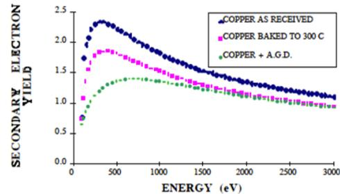
Figure 5: The SEY data of different copper surfaces [6].
