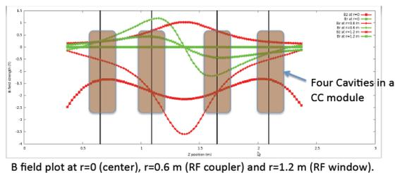
Figure 4: Magnetic field vector component  $B_r$  and  $B_z$  plot in CC module.
