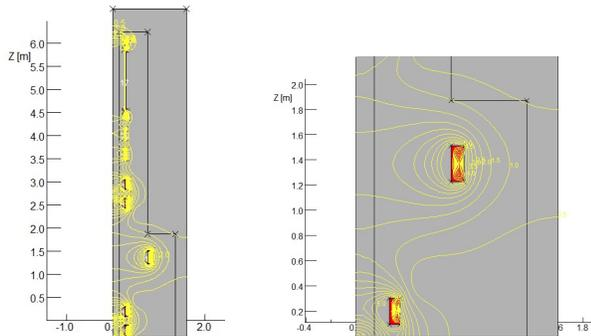
Figure 3: The magnitude contour plot of the magnetic field of solenoid mode in the MICE cooling channel. The left figure shows the field mapping in half of the whole channel. The right figure is a close-up view of the magnetic field distribution in the RFCC module, where the RF cavities are to be installed.
